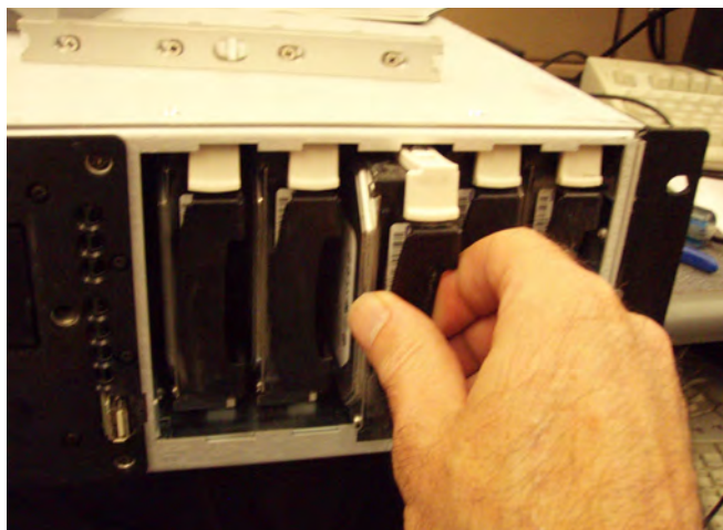
Figure 11 Slide Replacement Drive into Slot
