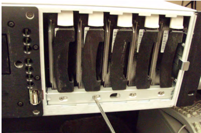
Figure 12 Reinstall Retaining Bracket
