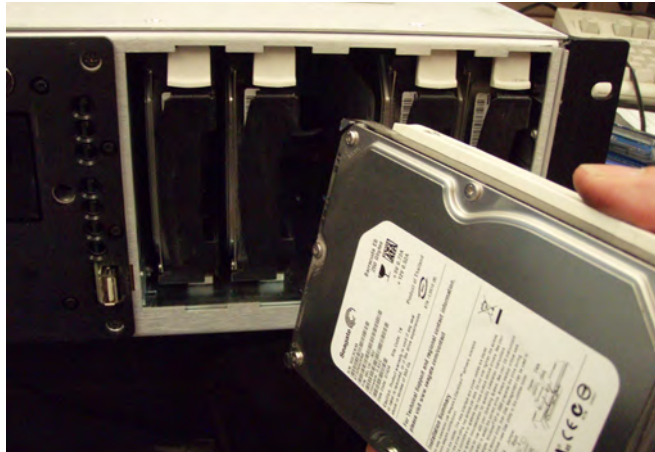
Figure 10 Grasp Replacement Drive's Finger Tab
