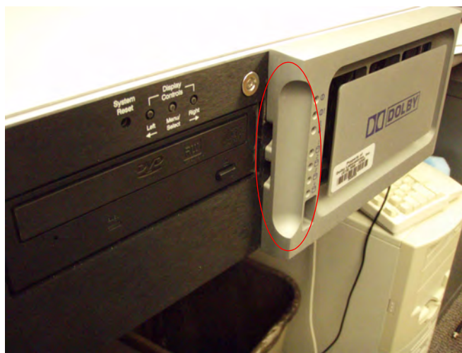
Figure 3 Locate Pry Areas Behind Right Panel
