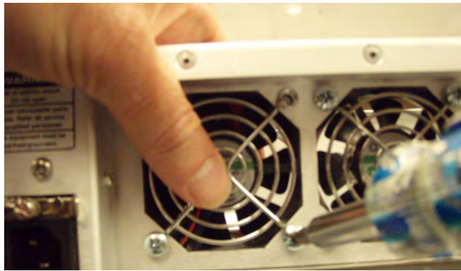
Figure 12 Install Replacement Fan in Unit and Replace Screws
