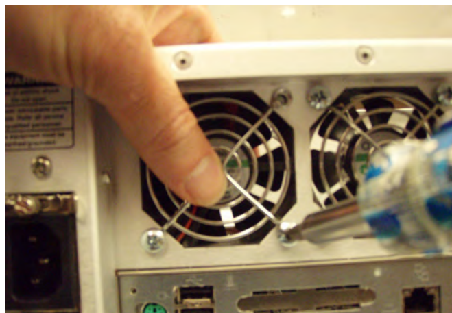
Figure 9 Remove Four Fan Screws
