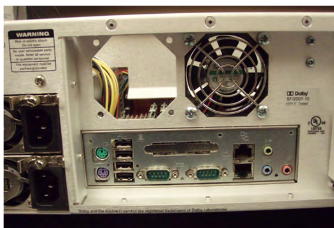
Figure 10 Remove Failed Fan Assembly
