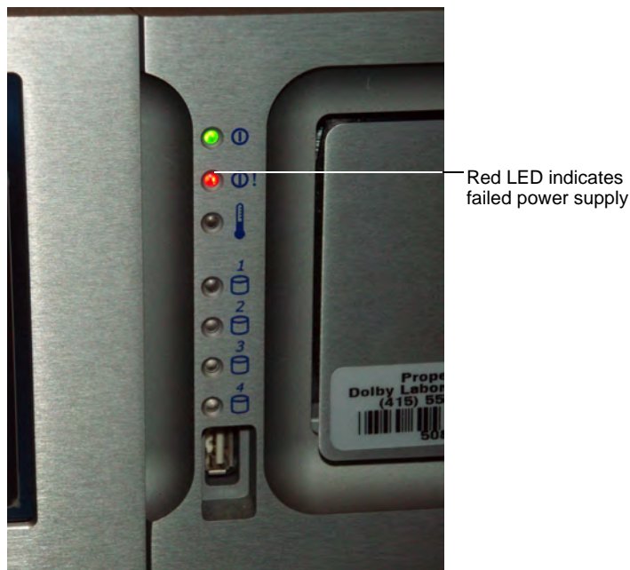
Figure 1 Red LED on Front Panel Indicates Failed Power Supply
