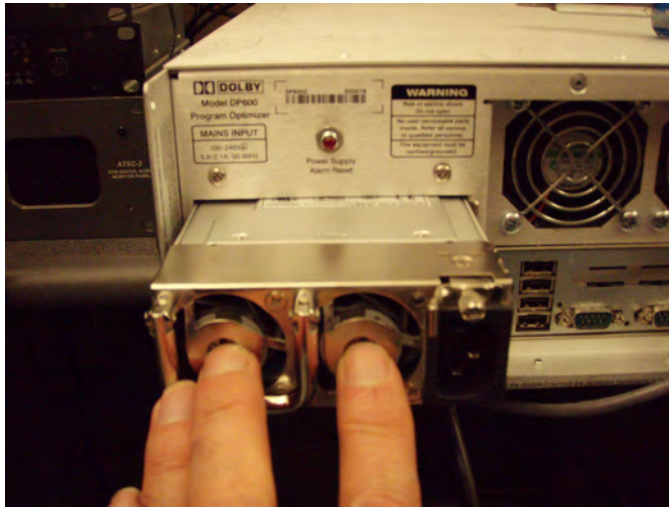
Figure 6 Slide Replacement Unit into Vacant Bay
