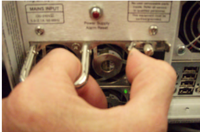
Figure 4 Grasp Handle on Failed Power Supply
