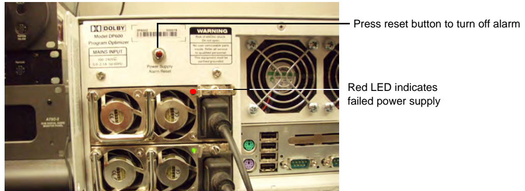
Figure 2 Locate Failed Power Supply
