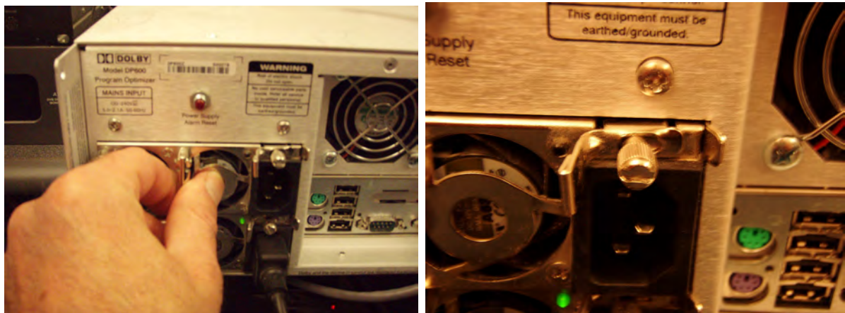
Figure 7 Push In Replacement Unit
