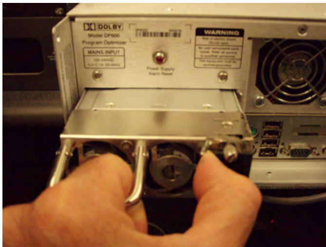
Figure 5 Remove Failed Power Supply
