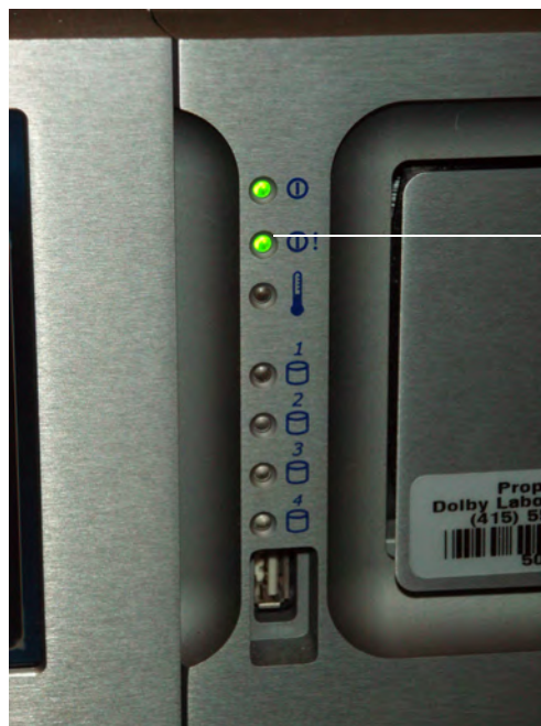
Figure 9 Green LED Indicates Functioning Power Supply
