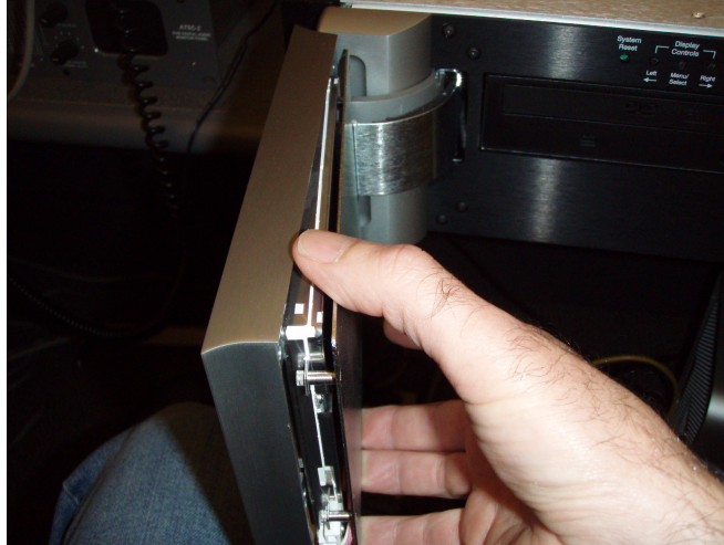
Figure 11 Reinstall Support Panel with New Touch Screen into Front-Panel Window
