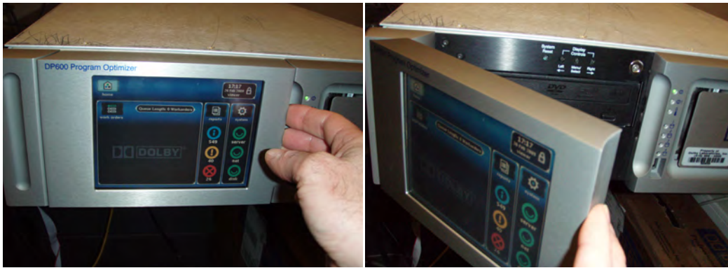
Figure 3-2 Swing Out Touch-Screen Panel
