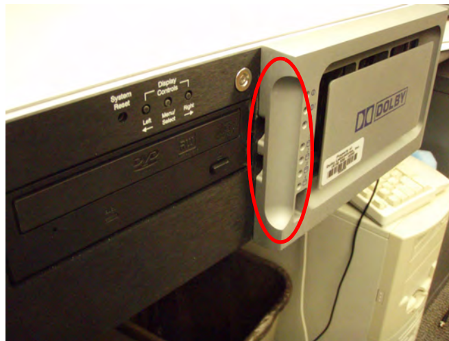
Figure 3-3 Locate Pry Areas Behind Drive Cover
