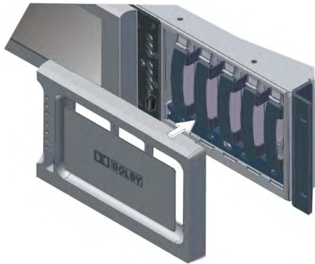
Figure 3-10 Reinstall Front-Panel Drive Cover
