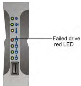
Figure 3-1 Red LED Indicates Failed Disk Drive
