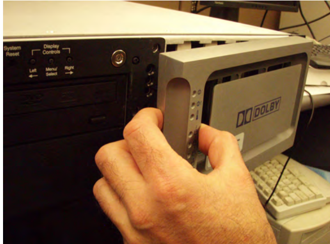
Figure 3-4 Remove the DP600 Drive Cover
