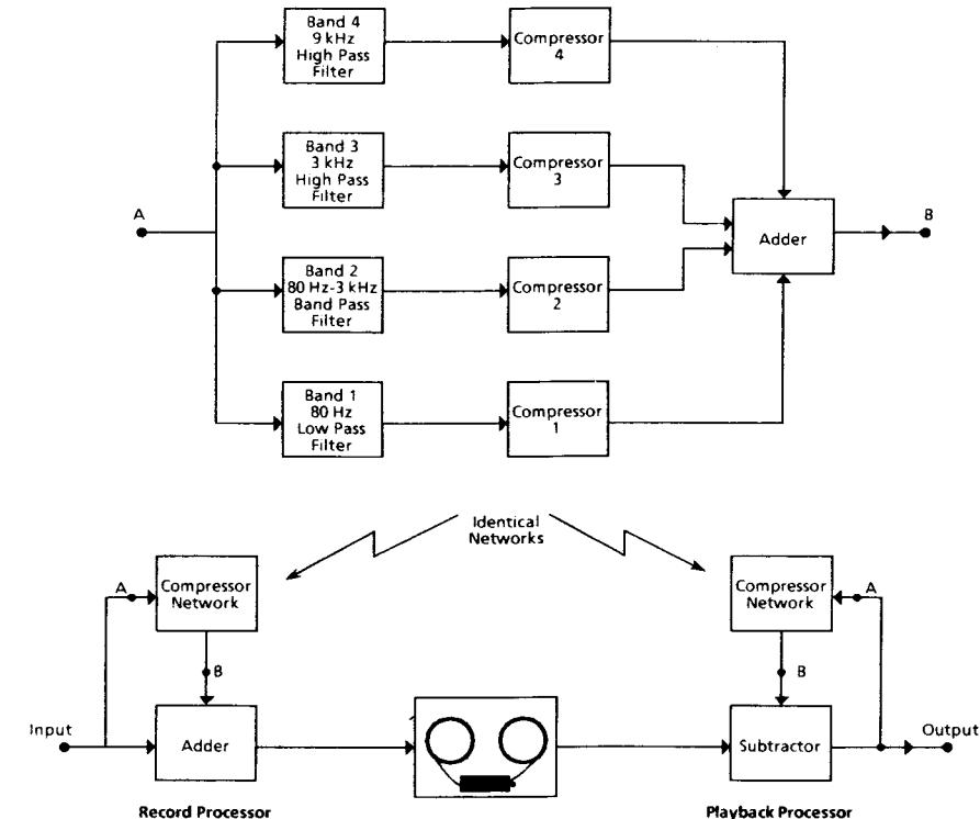
Noise Reduction System - Basic Block Diagram
