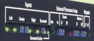
**The Dolby SEU4 is for use during soundtrack production to encode discrete four-channel program material for Dolby Surround release.**
